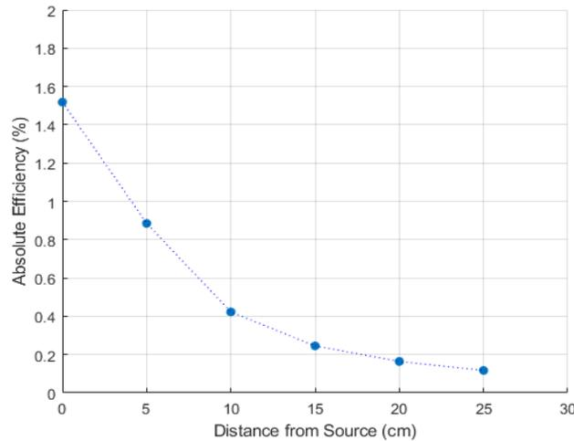
**Figure 6.** Distance dependence plot. Radioactive source:  $^{137}\text{Cs}$  (662 keV)
