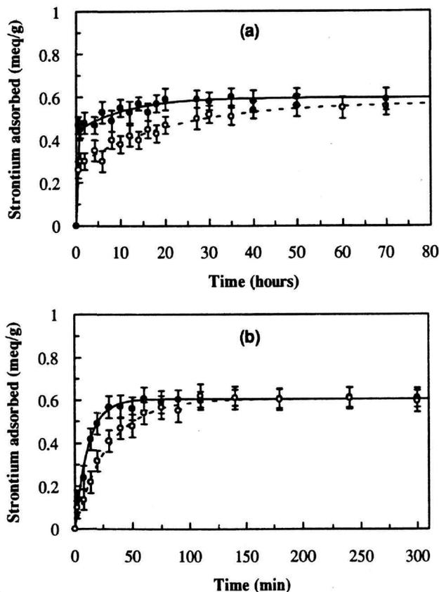
Fig.3 Sr<sup>2+</sup> exchange kinetics on FRAZA-D (black circles, solid curves) and AZA-D (open circles, dashed curves) under (a) static and (b) dynamic experimental conditions.
