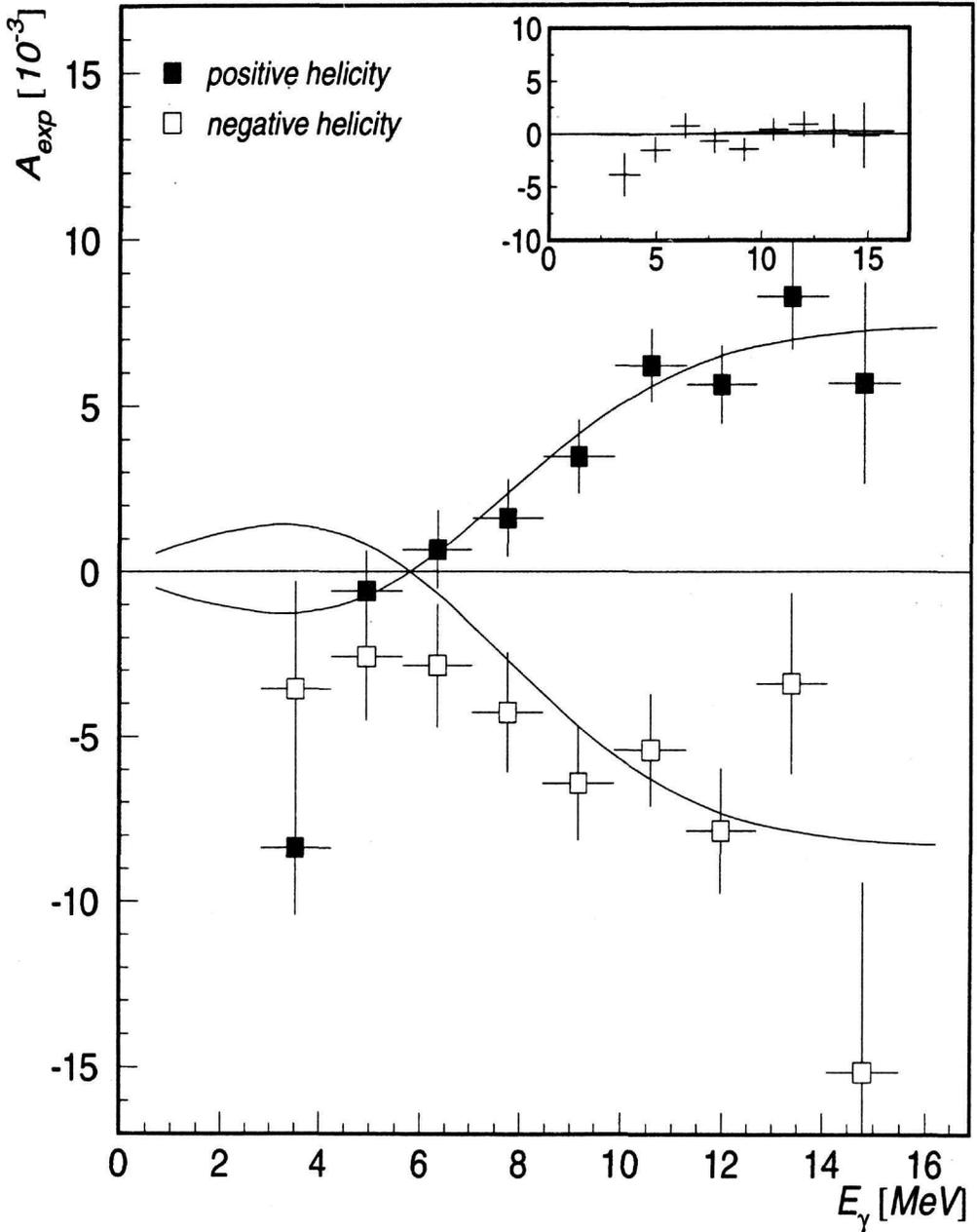
Fig.2 Experimental asymmetries  $A_{exp}$  as a function of the energy of the backscattered photons ( $E_\gamma$ ) for positive and negative electron helicity and for unpolarized electrons (inset). The line is the best fit of  $P_z < \alpha_{3z}(E_\gamma) >$  to  $A_{exp}$ .
