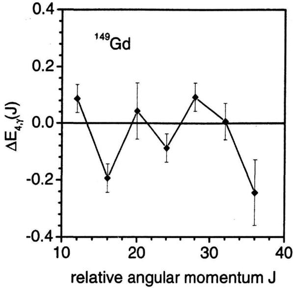
Fig. 4.  $\Delta J = 4$  staggering for the superdeformed band (a) of the  $^{149}\text{Gd}$  nucleus. (Data from [6].) Since no final angular momentum assignments have been made for this spectrum, angular momentum is measured relative to the lowest observed level of the superdeformed band.
