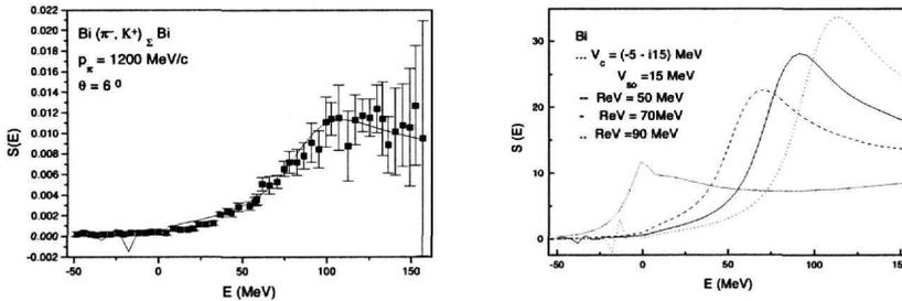
Fig. 4. a. The calculated spectrum for  $V_c = (80, -i23) MeV$ ,  $V_{so} = 25 MeV$  for the KEK experiment for  $\Sigma Bi(\pi^-, K^+)$  together with the experimental spectrum [10]. b. The calculated spectra for the KEK experiment [10] for  $\Sigma Bi(\pi^-, K^+)$  when  $ReV_c$  takes the values: -5, 50, 70, 90 MeV from the left to the right respectively and  $ImV_c = -15 MeV$ ,  $V_{so} = 15 MeV$ .
