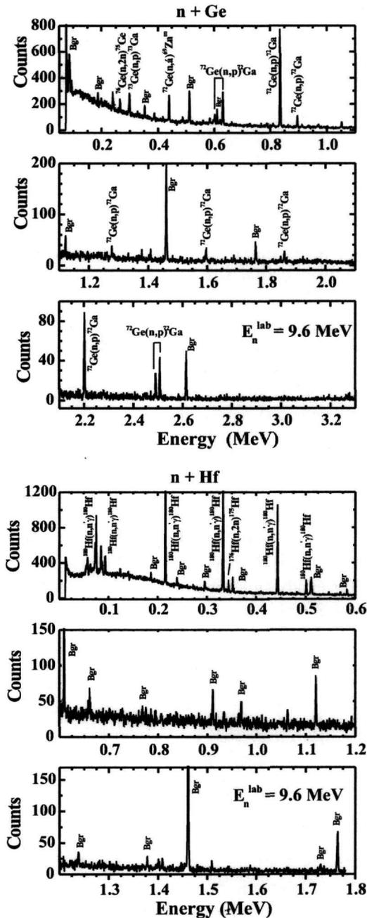
Fig. 2. Typical neutron activation spectra from isotopes of natural Ge and Hf.
