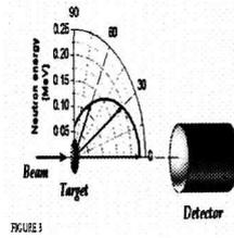
Fig. 2. Arrangement of the detector in respect to the beam direction. Neutron energy as a function of the emission angle is also presented for the case of  ${}^7\text{Li}(p,n){}^7\text{Be}$  reaction when proton energy is 2 MeV, as an example.
