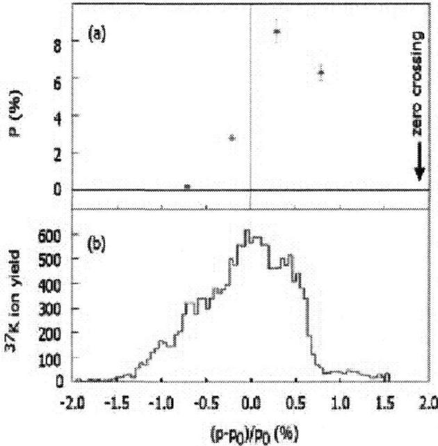
Fig. 2. Spin polarization of  $^{37}\text{K}$  vs. the momentum distribution.
