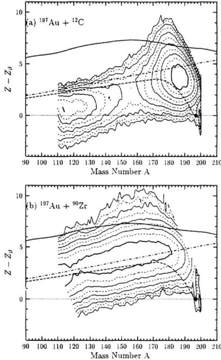
Fig. 3. Fragment yield distributions as a function of  $Z$  (relative to the line of  $\beta$  stability,  $Z_\beta$ ) and  $A$  for the reaction of 30 MeV/nucleon  $^{197}\text{Au}$  with  $^{90}\text{Zr}$ . The dashed line indicates the expected values for relativistic nuclear collisions [12], the dot-dashed line indicates the position of the “evaporation residue attractor line” [13] and the solid line indicates the average position of the proton dripline for odd  $Z$  nuclei [15].
