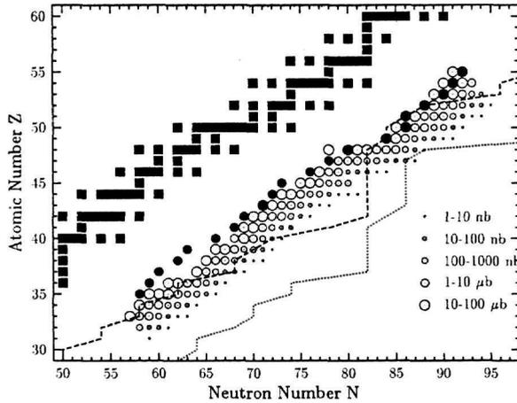
Fig. 10. Z-N plot displaying cross section estimates (open circles) of very neutron-rich nuclei from the interaction of 20 MeV/nucleon  $^{238}\text{U}$  with  $^{208}\text{Pb}$ . Stable nuclei are shown with squares. The solid circles are the most n-rich nuclides produced in the experiment. The dashed line shows a typical r-process path and the dotted-line shows the position of the odd-Z neutron drip-line (lines taken from Ref. [15]).
