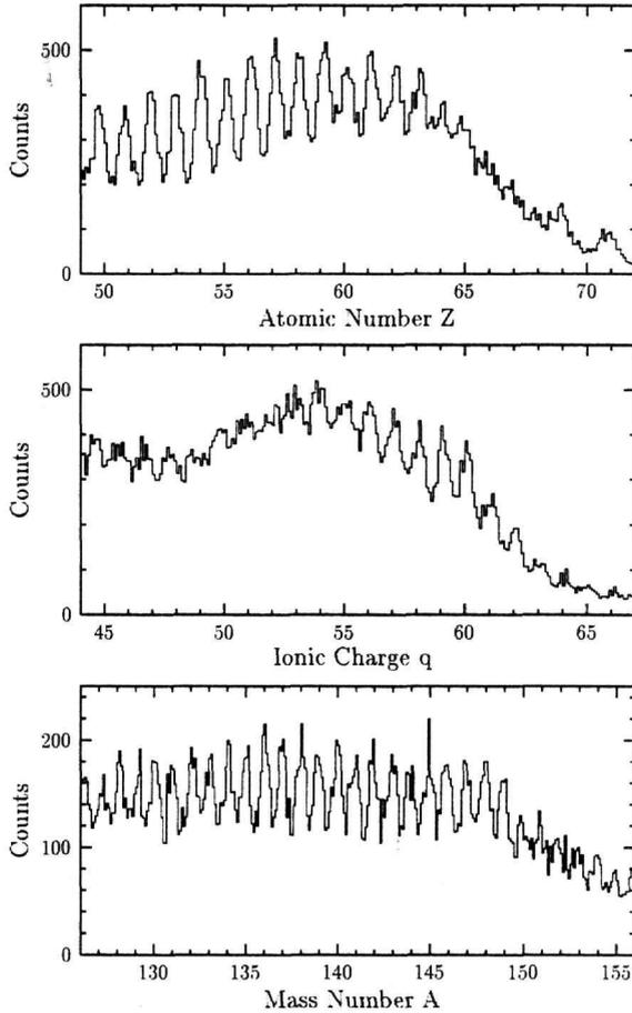
Fig. 1. Typical examples of the Z, q and A spectra of heavy fragments from the reaction of 30 MeV/nucleon  $^{197}\text{Au} + ^{90}\text{Zr}$ .
