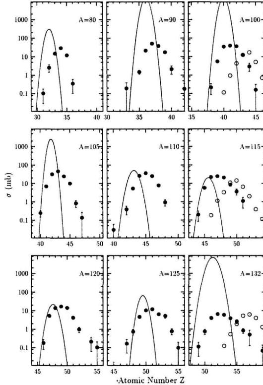
Fig. 9. Charge distributions for representative nuclei formed in the 20 MeV/nucleon  $^{238}\text{U} + ^{208}\text{Pb}$  reaction. Also shown are similar data for thermal neutron induced fission of  $^{235}\text{U}$  (solid lines) and the 20 MeV/nucleon  $^{238}\text{U} + ^{27}\text{Al}$  reaction [6] (open circles).
