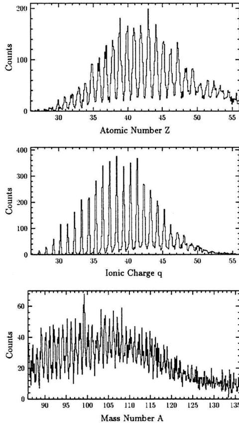
Fig. 6. Typical examples of measured  $Z$ ,  $q$  and  $A$  distributions for fission fragments from the reaction of 20 MeV/nucleon  $^{238}\text{U}$  with  $^{208}\text{Pb}$  at a single spectrometer setting.
