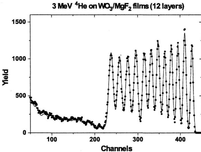
Fig. 2. RBS spectrum of 12 layer pairs of  $\text{WO}_3/\text{MgF}_2$  films on UV glass taken with 3 MeV  $^4\text{He}$ . The 12 strong peaks of W correspond to the 12 layers of  $\text{WO}_3$ . The solid line represents simulation by the RUMP code.
