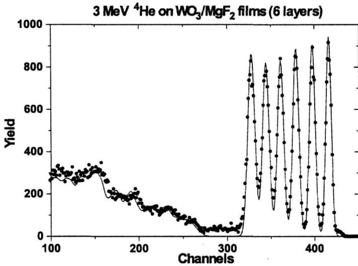
Fig. 1. RBS spectrum of 6 layer pairs of  $\text{WO}_3/\text{MgF}_2$  films on UV glass taken with 3 MeV  $^4\text{He}$ . The 6 strong peaks of W correspond to the 12 layers of  $\text{WO}_3$ . The solid line represents simulation by the RUMP code.
