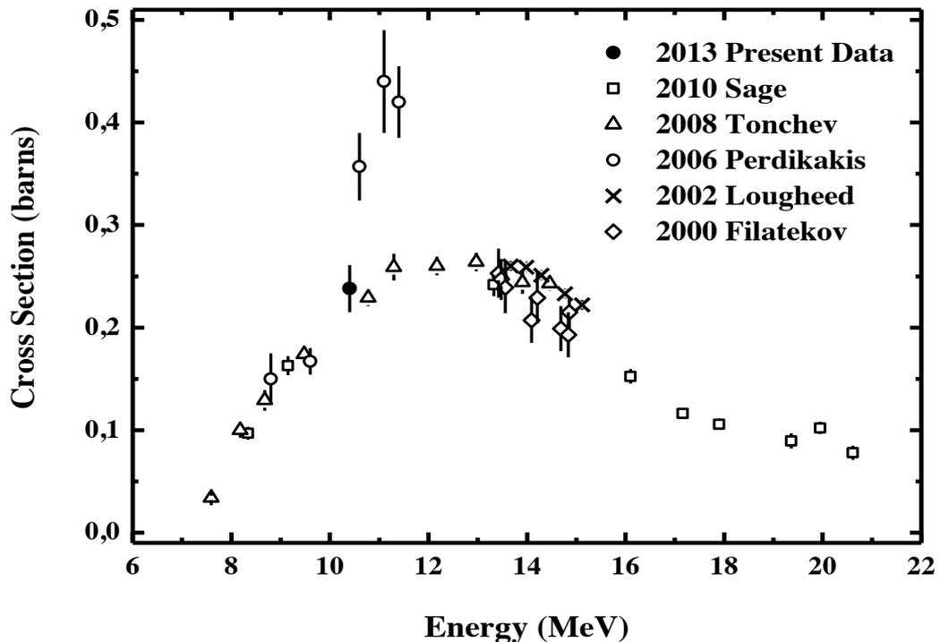
Fig. 1. Cross section of the  $^{241}\text{Am}(n,2n)$  reaction
