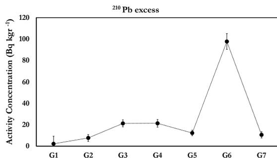
Figure 5: <sup>210</sup>Pb excess activity concentration in sediment samples at the points G1-G7.
