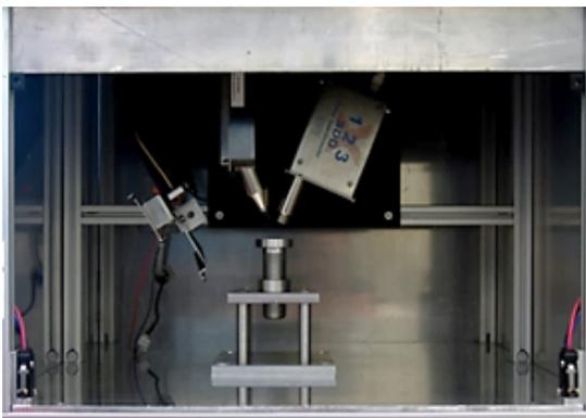
Figure 1: EDXRF system located at NCSR “Demokritos”
