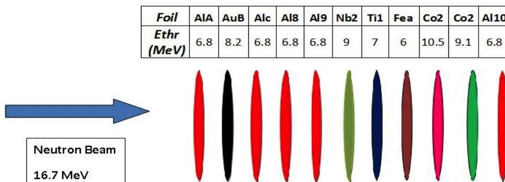
Figure 2: The foil assembly irradiated with the 16.7 MeV neutron beam
