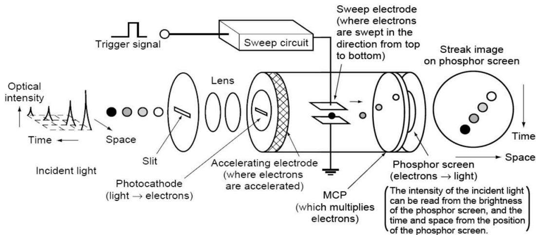
Figure 3: Streak Camera: Principle of Operation.
