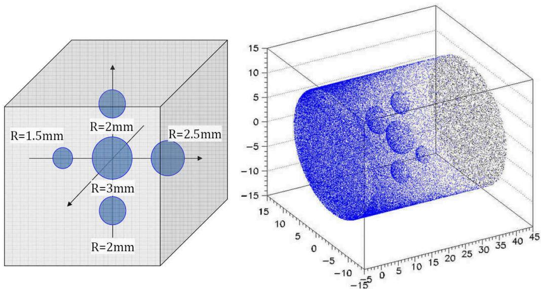
Figure 4: Geometry of the optical phantom with five refractive spheres in an air cylinder used in the Monte-Carlo simulation study with the DETECT2000 program. Absorbed and escaped photons during the simulation process are shown in the 3D plot. The light source is on the left side of the cylinder, while the detector resides on the right.
