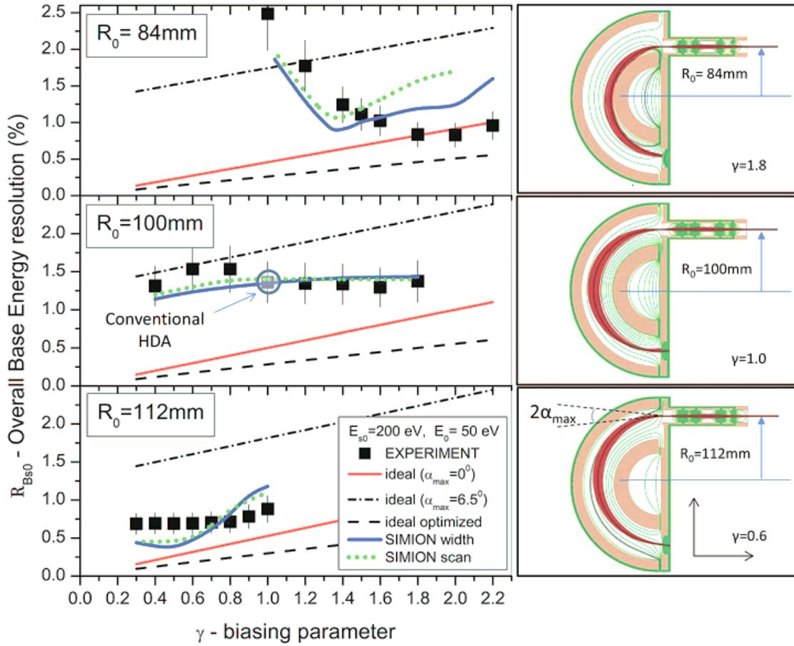
Figure 4: (Left) HDA overall base resolution  $R_{B_{s0}}$  plotted as a function of the biasing parameter for experimental, simulation and theoretical calculations for the 3 positions of the lens. (Right) Respectively, the schematics of SIMION simulations in the  $Y=0$  dispersion plane of the spectrometer for conventional and paracentric positions. Electron trajectories are shown in red and equipotentials in green.
