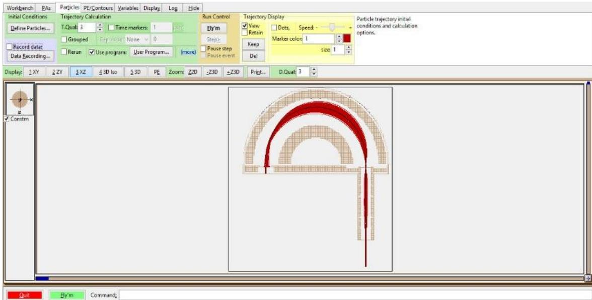
Figure 3: The SIMION workbench where all variables can be adjusted so as to start flying the particles. Automation coding is also supported, which can save a significant amount of time by running multiple simulation conditions at once.
