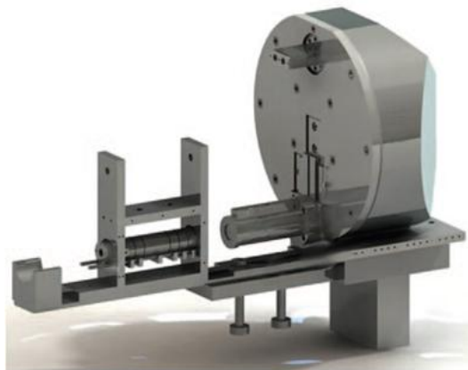
Figure 1: The actual setup of the analyser in 3D. The HDA and movable lens are enclosed in an insulated shell. In front of the lens is the electron gun.
