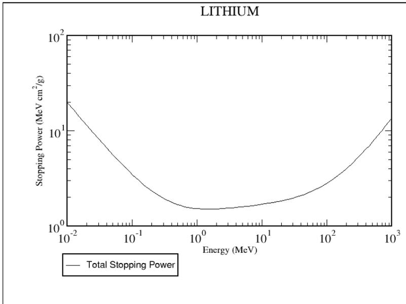
Figure 4. The stopping power of electrons in Lithium.
