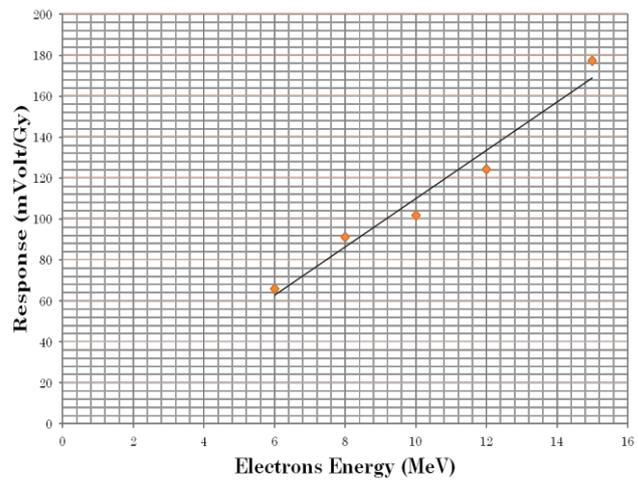
Figure 3. The Linearity of the dose response as a function of the energy of the electron beam.
