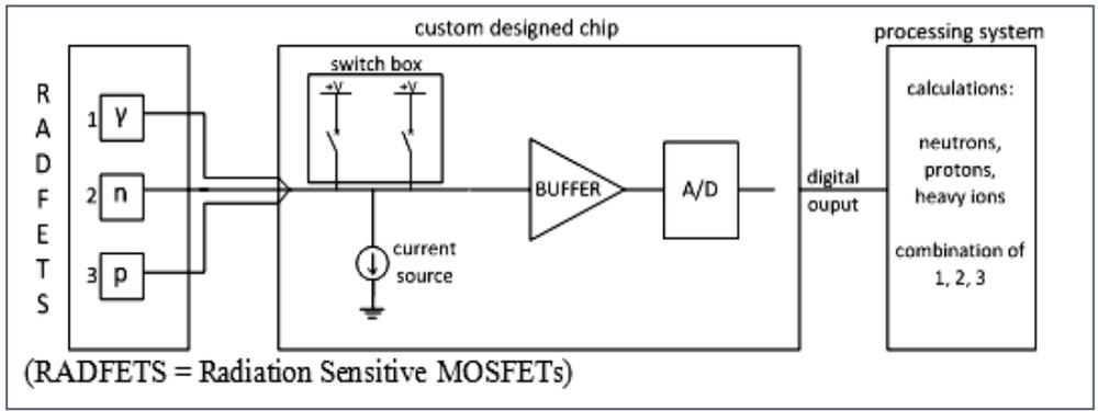
Figure 1. A block diagram of the complete system
