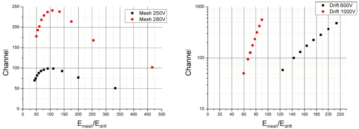
Figure 2: The transparency curve (left) and the gain curve (right) obtained from the testing of one of the microbulks used. The peak at the transparency is reached when  $E_{\text{mesh}}/E_{\text{drift}} \sim 110$ .
