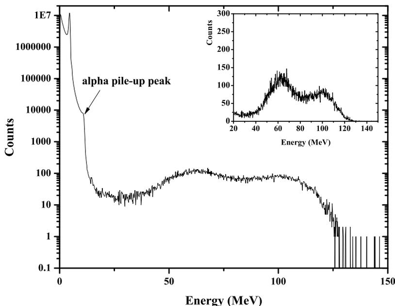
Figure 4: A typical spectrum obtained for the  $^{237}\text{Np}$  target in logarithmic scale. The high alpha activity is causing pile-up effect, however orders of magnitude lower than the main peak. The inset contains the same spectrum zoomed at the fission fragment pulses, in a linear scale. The picture is taken from [5].
