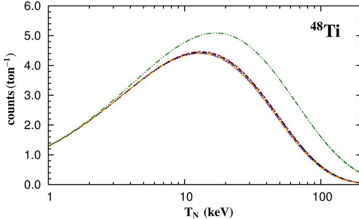
Figure 4: The response function for a terrestrial nuclear detector that consists of 1 tone  $^{48}\text{Ti}$ .
