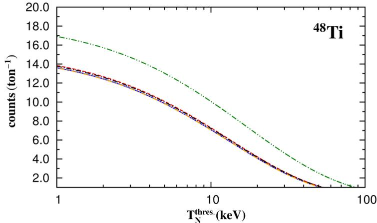
Figure 5: Number of total counts over threshold for a nuclear detector filled with 1 tone  $^{48}\text{Ti}$ .
