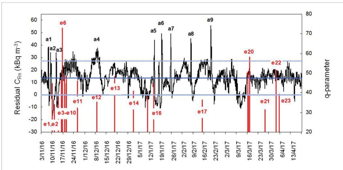
**Fig. 2.** Residual soil radon concentrations after correction for the atmospheric pressure effect. The average and  $\pm 2\sigma$  deviation values are shown in blue lines. The observed radon anomalies ( $a_i$ ) are compared with earthquakes ( $e_i$ ) from Table 1.
