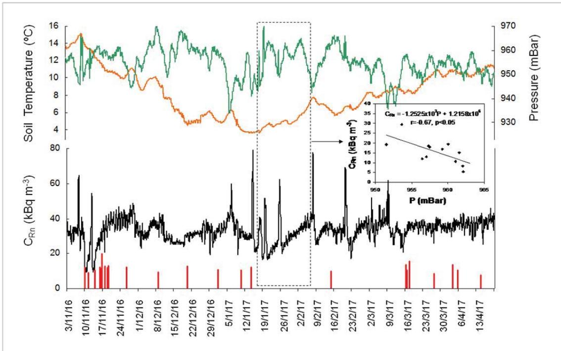
**Fig. 1.** Temporal fluctuation of soil radon concentration ( $C_{Rn}$ ), soil temperature and atmospheric pressure. Seismic events are indicated by red lines, corresponding to their  $q$ -parameter (see text). Inset: The linear regression model applied to account for the effect of atmospheric pressure on radon variation.
