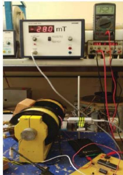
**Fig. 3.** The experimental setup, made by a dc power supply set to 15.5 V connected to the controller, which supplies the electromagnet. Using a magnetic probe the magnitude is measured with the teslameter. A slight voltage drop due to circuit resistance is apparent in the multimeter.
