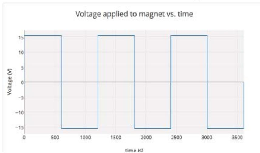
**Fig. 4.** Applied voltage time series. Field was flipped every 10 min with a 1 s zero-voltage interval to allow for reaching the hysteresis curve plateau.
