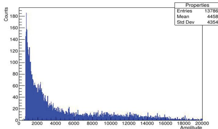
**Fig. 3.** Amplitude histogram for thermal and fast neutrons
