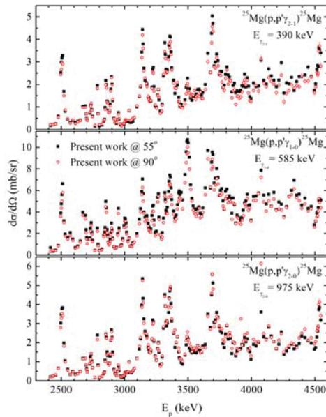
**Fig. 2.** Differential cross sections of the  $^{25}\text{Mg}(p,p'\gamma)^{25}\text{Mg}$  reaction for the two detection angles ( $55^\circ$  and  $90^\circ$ ) and the 390, 585 and 975 keV  $\gamma$ -rays emitted (top to bottom, respectively).
