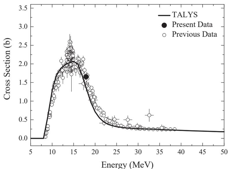
**Fig. 3.** Cross section theoretical calculations for the  $^{197}\text{Au}(n,2n)^{196}\text{Au}$  reaction obtained with TALYS 1.8 code, along with the data point of this work at 17.9 MeV and EXFOR data [5].
