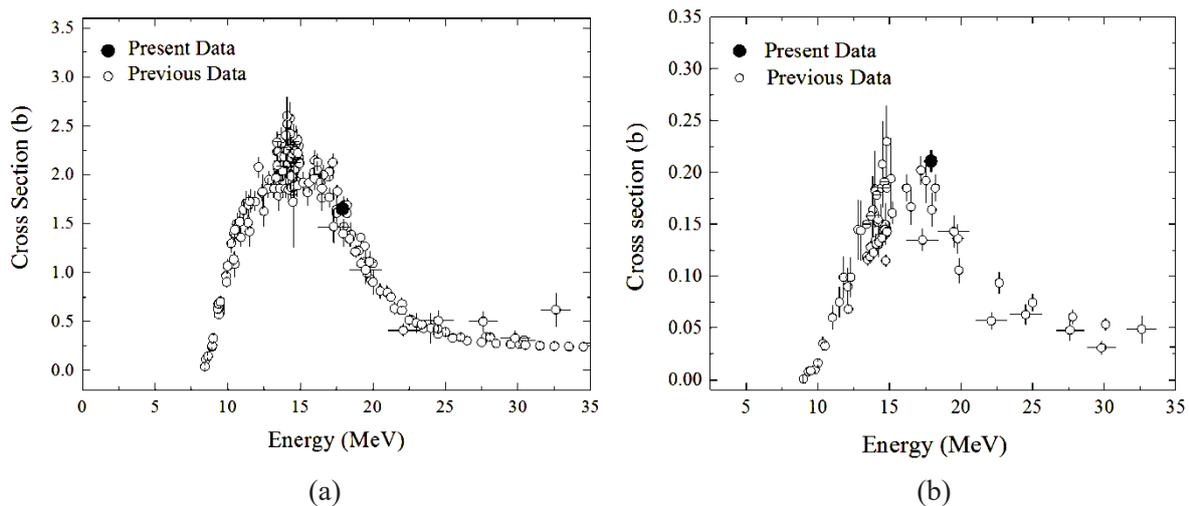
**Fig. 2.** Preliminary cross section values, along with the existing experimental data in literature [5], for (a) the  $^{197}\text{Au}(n,2n)^{196}\text{Au}$  reaction, (b) the  $^{197}\text{Au}(n,2n)^{196}\text{Au}^{m2}$  reaction
