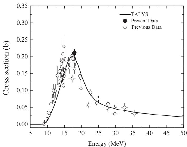
**Fig. 4.** Cross section theoretical calculations for the  $^{197}\text{Au}(n,2n)^{196}\text{Au}^{m2}$  reaction obtained with TALYS 1.8 code, along with the data point of this work at 17.9 MeV and EXFOR data [5].
