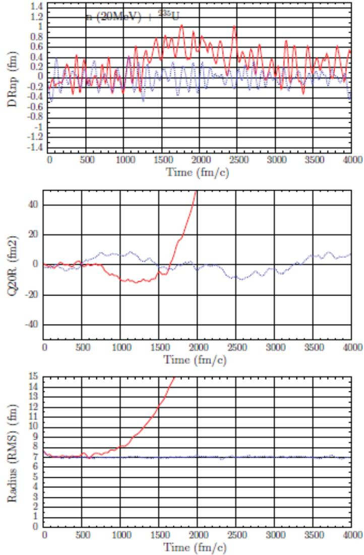
**Fig. 2.** (Color online) CoMD calculations on important macroscopic quantities of the nucleus versus time for the reaction  $n(20\text{MeV})+^{235}\text{U}$ . Red continuous line: Calculation with  $C_s=0$ . Blue dotted line: Calculation with  $C_s=-2$ . a) Relative distance between the centres of mass of protons and neutrons (GDR). b) Time evolution of the quadrupole moment (GQR). c) Time evolution of the radius (GMR).
