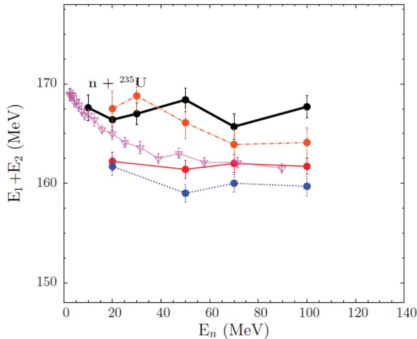
**Fig. 5.** (Color online) CoMD calculations on average total energy of fission fragments with respect to incident neutron energy. Red points connected with thin dotted lines: CoMD calculations with standard symmetry potential and  $Cs=0$ . Blue points connected with dotted line: CoMD calculations with soft symmetry potential and  $Cs=0$ . Black points: CoMD calculations with standard symmetry potential and  $Cs=-2$ . Pink open triangles: experimental data of the Loveland group [1].
