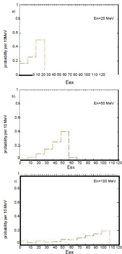
**Fig. 3.** (Color online) CoMD calculations on the distribution of the excitation energy of the compound nucleus at 3000 fm/c. a) probability of the excitation energy for the reaction  $n(20 \text{ MeV})+^{235}\text{U}$ . b) probability of the excitation energy for the reaction  $n(50 \text{ MeV})+^{235}\text{U}$ . c) probability of the excitation energy for the reaction  $n(100 \text{ MeV})+^{235}\text{U}$ .
