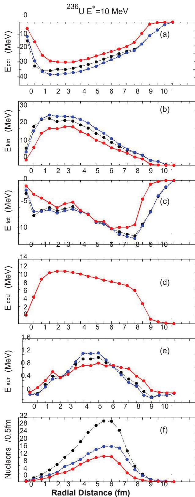
**Fig. 1.** (Color online) Calculated energy terms per nucleon versus radial distance. Red line: protons. Blue line: neutrons. Black line: nucleons. a) Potential energy per nucleon. b) Kinetic energy. c) Total energy. d) Energy Coulomb. e) Surface energy. f) Nucleons/0.5 fm.
