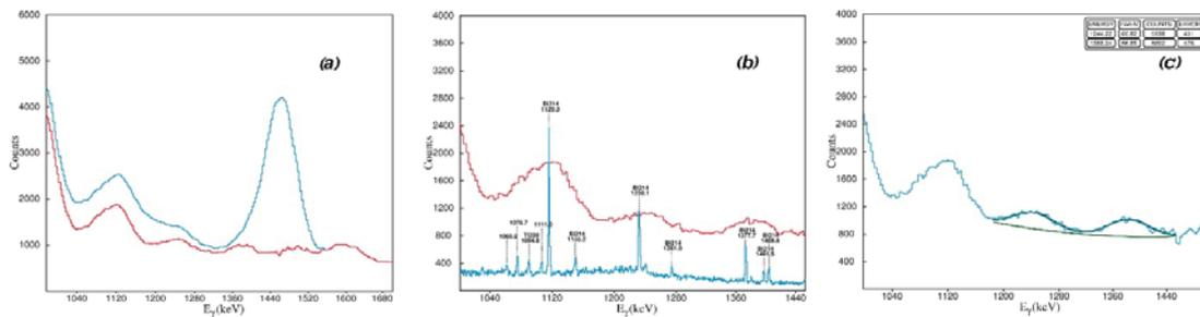
**Fig. 3.** a) Partial NaI spectrum before and after subtracting  $^{40}\text{K}$ , b) The HPGGe and NaI spectra in the region of 1120-1380 keV, c) Evaluation of the number of net counts in the 1238+1281 and 1378 peaks.
