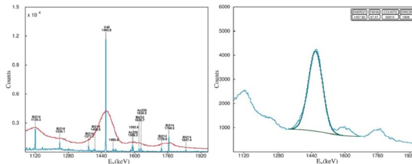
**Fig. 4.** The HPGGe and NaI spectra in the region of 1460 keV and the evaluation of the 1460 photo-peak
