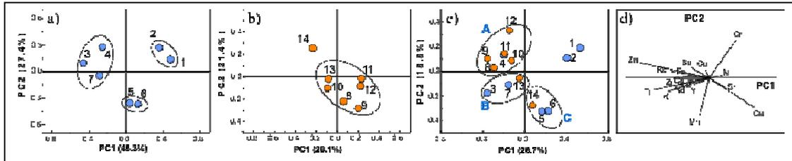
**Fig. 4.** (a) A PC1-PC2 score plot for samples collected from the upthrown fault block. (b) A PC1-PC2 score plot for samples collected from the downthrown fault block. (c) A PC1-PC2 score plot for the entire sample set (blue: upthrown fault block; orange: downthrown fault block). (d) Elemental loadings' plot indicating the effect of the elemental variables on the PC1-PC2 coordinates of the samples.
