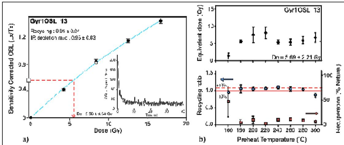
Fig. 3. (a) Typical dose-response curve and natural OSL signal decay curve (inset) from sample Gyr1OSL\_13. (b) Preheat plateau test results showing the lack of dependence of equivalent dose, recycling ratio and recuperation on preheat temperature for sample Gyr1OSL\_13. Each point represents the average of results from three aliquots.
