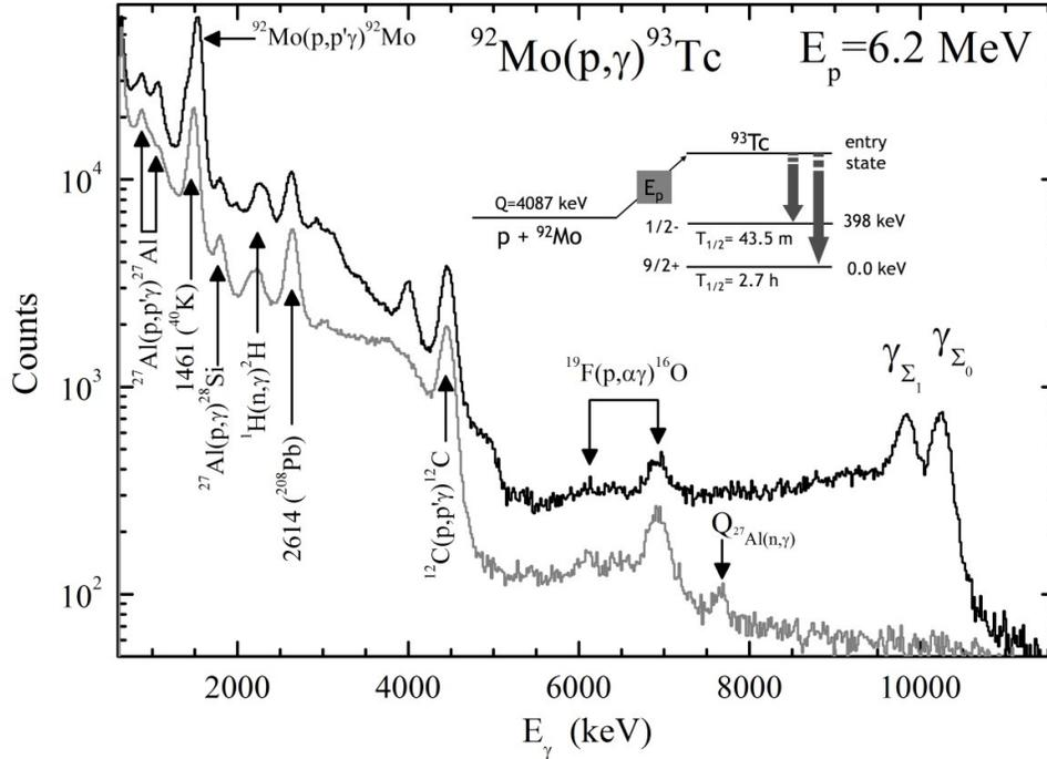
Fig. 1: Typical spectrum of the  $^{92}\text{Mo}(p,\gamma)^{93}\text{Tc}$  reaction measured at  $E_p=6.2$  MeV with a  $4\pi$ -summing detector. A metastable state of the produced nucleus  $^{93}\text{Tc}$  at 392 keV results in the second peak  $\gamma_{\Sigma_1}$ .
