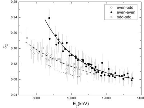
**Fig 2:** Sum-peak efficiencies determined by a systematic study using the method described in [3,4] for several capture reactions. The continuous lines correspond to fits of the exponential function, see text for more details, according to the type (even-even, even-odd or odd-odd) of the formed compound nucleus.
