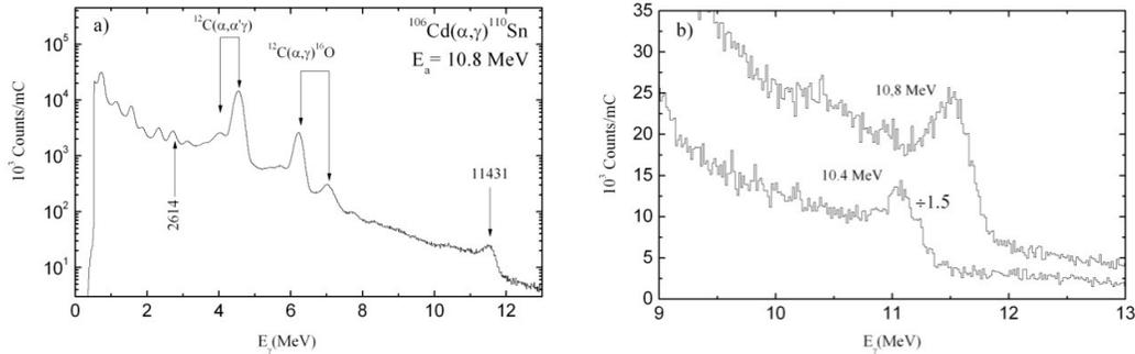
**Fig 1:** (a) Typical measured spectrum of  $4\pi$  angle integrated  $\gamma$ -singles for the reaction  $^{106}\text{Cd}(\alpha,\gamma)^{110}\text{Sn}$  at  $E_a=10.8$  MeV using the  $\gamma$ -summing NaI(Tl) crystal, (b) The same spectrum focused at the sum-peak energy range and a second one (scaled by a factor of 1.5) collected at  $E_a=10.4$  MeV.
