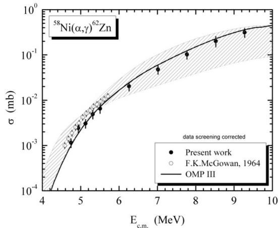
**Fig 3:** Comparison of experimental data of the reaction  $^{58}\text{Ni}(\alpha,\gamma)^{62}\text{Zn}$  obtained from the present work (solid circles). The cross sections obtained from [6] are denoted with open circles while the curve and the shaded area correspond to theoretical predictions calculated using the TALYS code, see text for more details.
