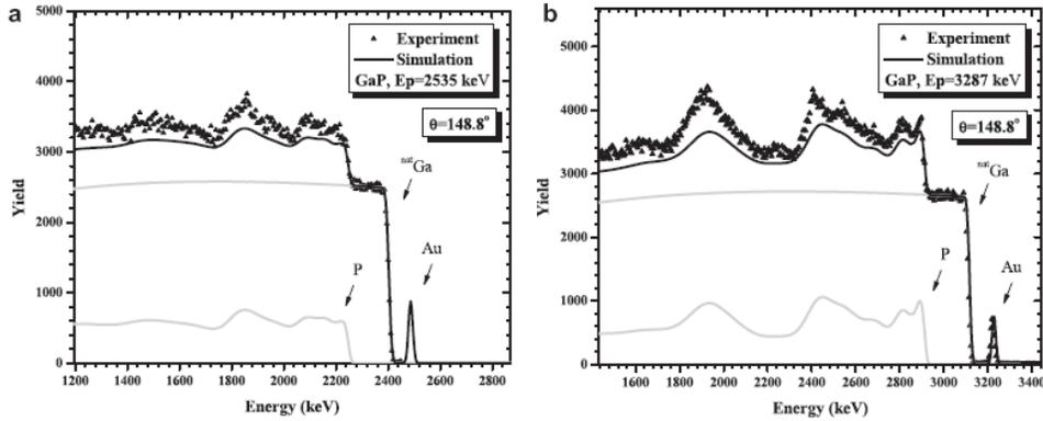
**Figures 8.** (a and b) Benchmarking results for  $^{31}\text{P}(p,p)$  at  $150^\circ$ , using the experimentally determined cross-section dataset by Karadzhev et al. [20] for the simulations at different beam energies.
