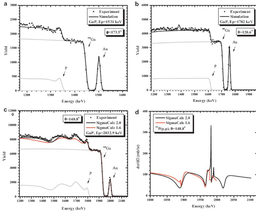
**Figures 7.** (a–c) Benchmarking results for  $^{31}\text{P}(p,p)$  using the corresponding evaluated cross-section datasets for the simulations at different beam energies and detection angles. (d) Comparison between the two versions of SigmaCalc.
