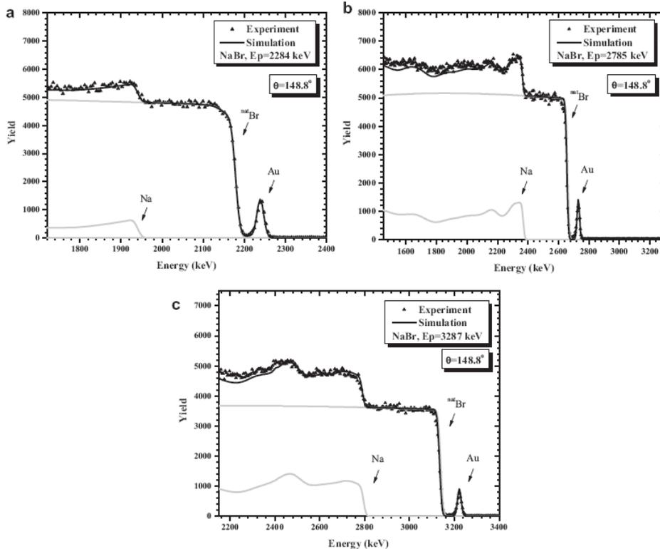
**Figures 6.** (a–c) Benchmarking results for  $^{23}\text{Na}(p,p)$  at  $150^\circ$ , using the experimentally determined cross-section dataset by Cacioli *et al.* [19] for the simulations at different beam energies.
