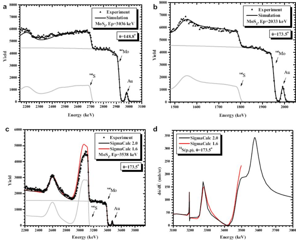
**Figures 4.** (a–c) Benchmarking results for  $^{nat}\text{S}(p,p)$  using the corresponding evaluated cross-section datasets for the simulations at different beam energies and detection angles. (d) Comparison between the two versions of SigmaCalc.
