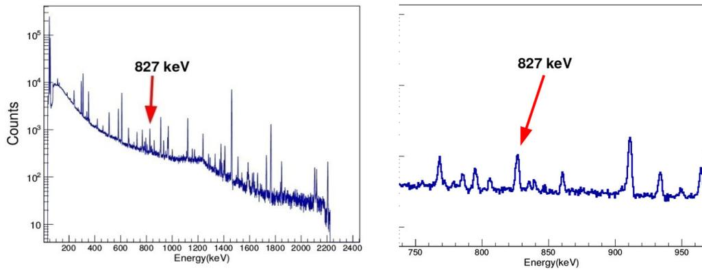
Figure 4: The  $\gamma$ -ray experimental spectrum of the Erbium sample after 10 h of irradiation 7h of activity measurement. The spectrum corresponds to the superposition of the spectra resulted from both HPGe that were previously gain matched. The right part is the enlargement of the region of interest around the strongest transition at 827 keV.
