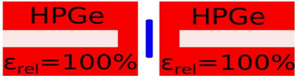
Figure 2: Erbium sample  $\gamma$ -ray measurements: Two HPGe detectors were used in close, face-to-face geometry. The sample (blue) to detector (red) distance was 1 cm. In this way, almost  $4\pi$  detection angle was covered resulting in 11% total peak efficiency for both HPGe detectors at the region of 830 keV.
