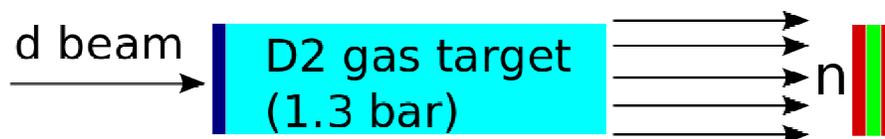
Figure 1: A simplified diagram of the irradiation setup. The neutron beam was produced by means of the  $\text{D}(d,n)^3\text{He}$  reaction. The sample sandwich was placed at  $0^\circ$  with respect the neutron beam.
