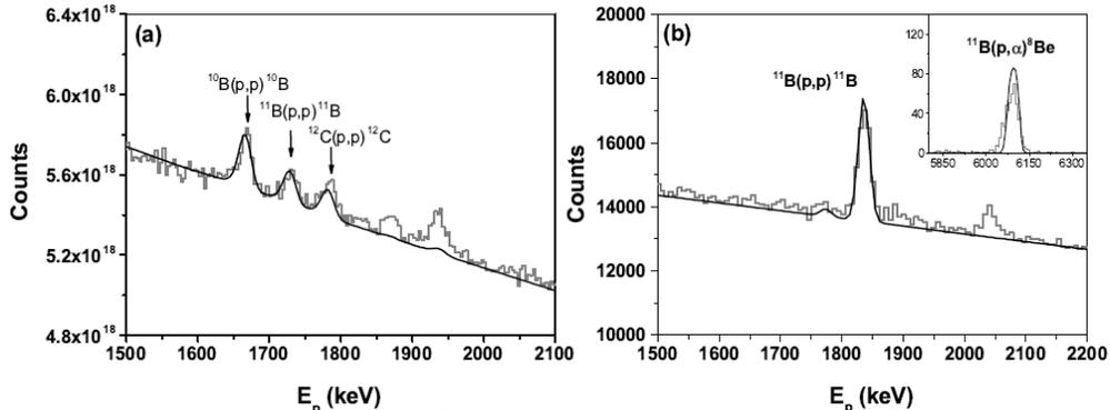
**Fig 1:** (a) The EBS spectrum of the  $^{10}\text{B}$  enriched target along with the simulation of SIMNRA [11]. The highly induced background from the Tantalum backing results at a high uncertainty in the determination of the target's thickness. (b) The backscattered elastic peak from  $^{11}\text{B}$  was analyzed simultaneously with the  $^{11}\text{B}(p,\alpha)^8\text{Be}$  peak (insert).
