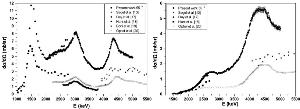
**Fig 3:** Comparison of the  $^{10}\text{B}(p,\alpha\gamma)^7\text{Be}$  and  $^{10}\text{B}(p,p'\gamma)^{10}\text{B}$  cross sections at  $55^\circ$  with the experimental data of previous works. The possible reasons for the observed differences are discussed in the text.
