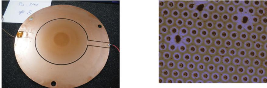
**Figure 1: Left:** One of the Micromegas detectors used with a  $^{240}\text{Pu}$  sample pictured after the end of the measurement. A 3 cm diameter discolouration is visible on the micromesh. **Right:** Picture of the micromesh taken with an electronic microscope. Mechanical damage around the rims of the holes can be observed. This leads to a severe deterioration of the detector gain and performance.
