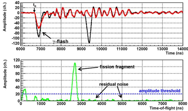
**Figure 2: Top:** The first few  $\mu\text{s}$  of the recorded signals during the same proton bunch from two adjacent detectors. The  $\gamma$ -flash signal and the baseline oscillations are clearly visible. **Bottom:** the residual signal after the subtraction of the two signals above. The oscillation is almost entirely suppressed.
