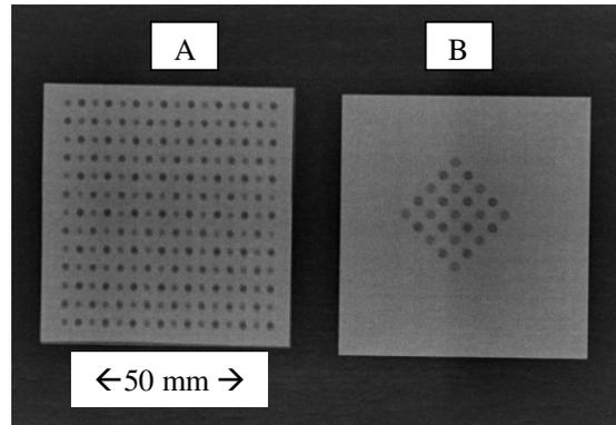
Fig. 1 X-ray image of C<sub>i</sub>/SiC samples analyzed in this work
