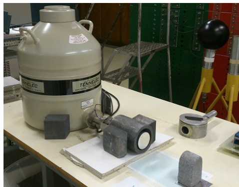
Figure 1: The \gamma -spectroscopy station with Pb shielding
