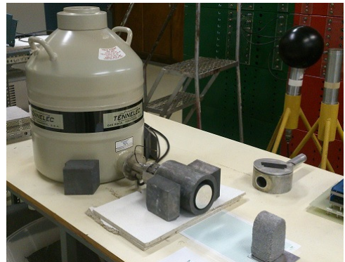
Figure 1: The \gamma -spectroscopy station with Pb shielding
