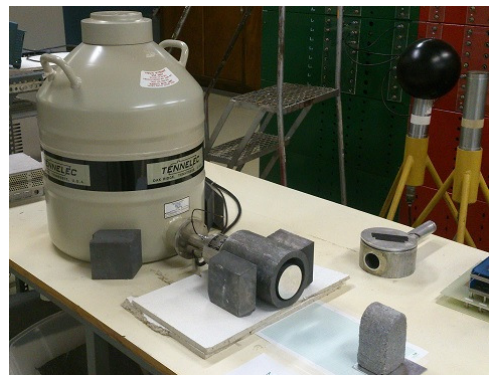
Figure 1: The \gamma -spectroscopy station with Pb shielding
