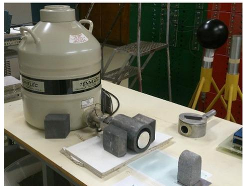
*Figure 1: The  $\gamma$ -spectroscopy station with Pb shielding*
