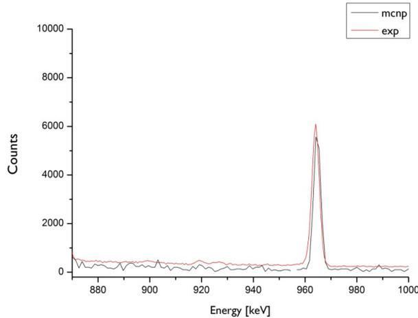
*Figure 5: Comparison of experimental data and simulation of the  $^{152}\text{Eu}$  at a distance of 10 cm from the detector for a randomly selected photopeak, after GEB was applied. The geometry resembles the real setup accurately as it is also evident by the off center placement of the hollow cylindrical Pb shield around the crystal.*
