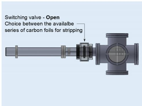
**Figure 2: Foil stripper sketch (in use).**
