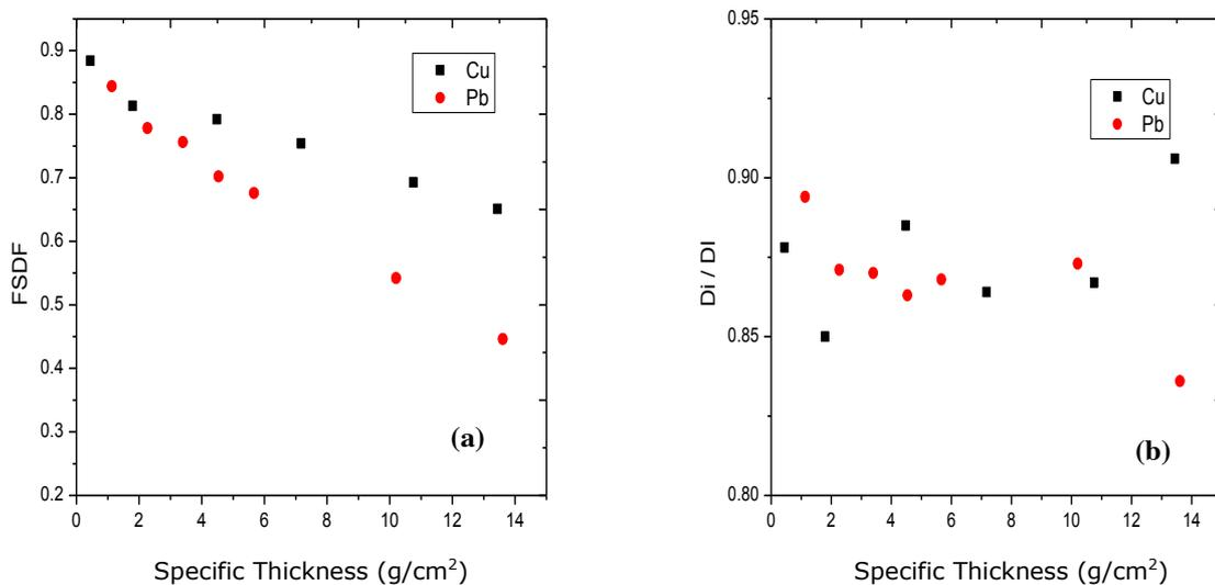
Figure 5: FSDF dependence on the specific thickness of the in-homogeneity with and without attenuation correction.
