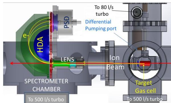
**Fig. 2.** Schematic view of the doubly-differentially pumped target gas cell, the 4-element input lens, the HDA and the 2-D PSD. Each colour denotes a different electrode that can be independently biased.
