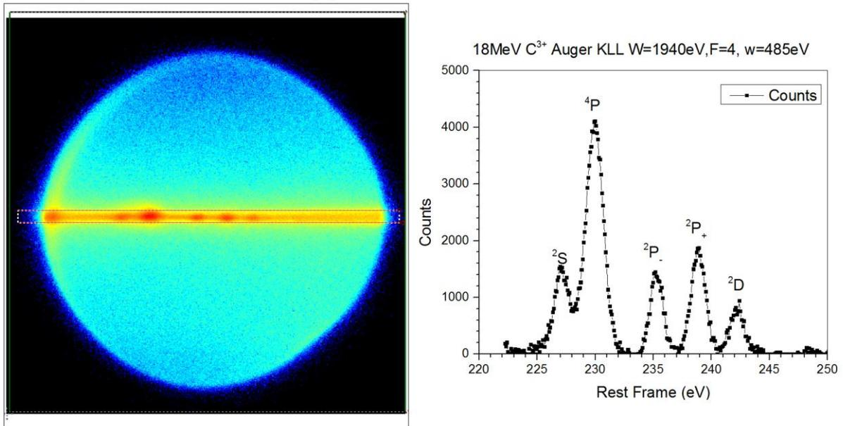
**Fig. 3.** (a) 2-D PSD Image, (b) Projection of the PSD image within the selected region shown in (a). The  $4P$  line is seen to be broadened. Its considerably longer life-time makes it decays closer to the spectrometer with increased angular acceptance and therefore kinematic broadening.
