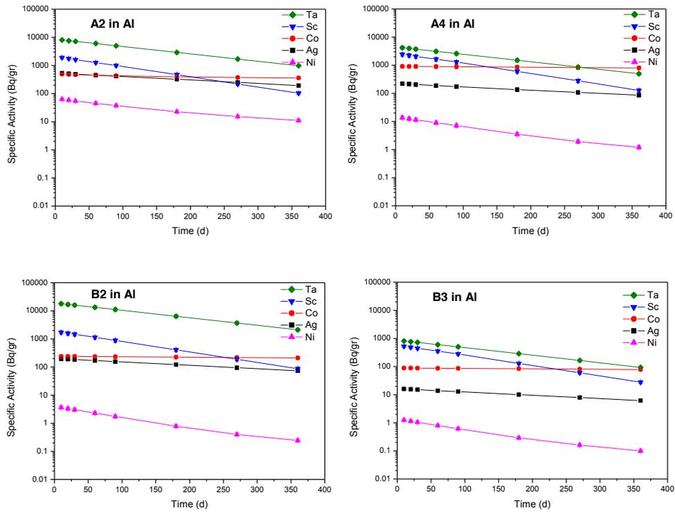
**Fig. 5** Predicted specific activity per foil within Al holders as a function of cooling time (D-T source)
