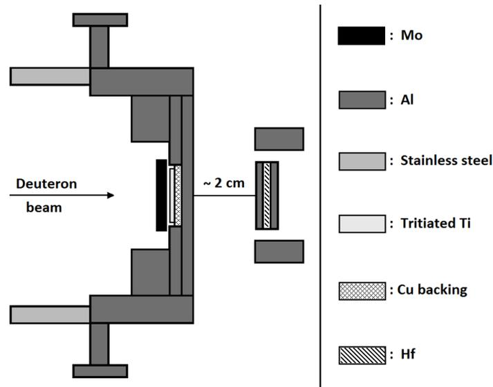
**Fig. 1.** Schematic representation of the irradiation setup geometry.
