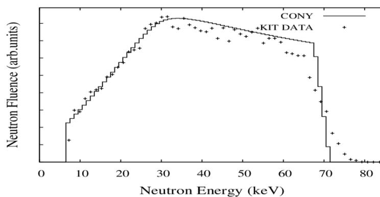
**Fig.2.** Experimental data from KIT. The neutron production (in arbitrary units) in comparison with CONY for  ${}^7\text{Li}(p,n){}^7\text{Be}$  for 1.892 MeV proton energy, thickness of natural lithium 30  $\mu\text{m}$  in thickness according to the detection geometry described in [12].
