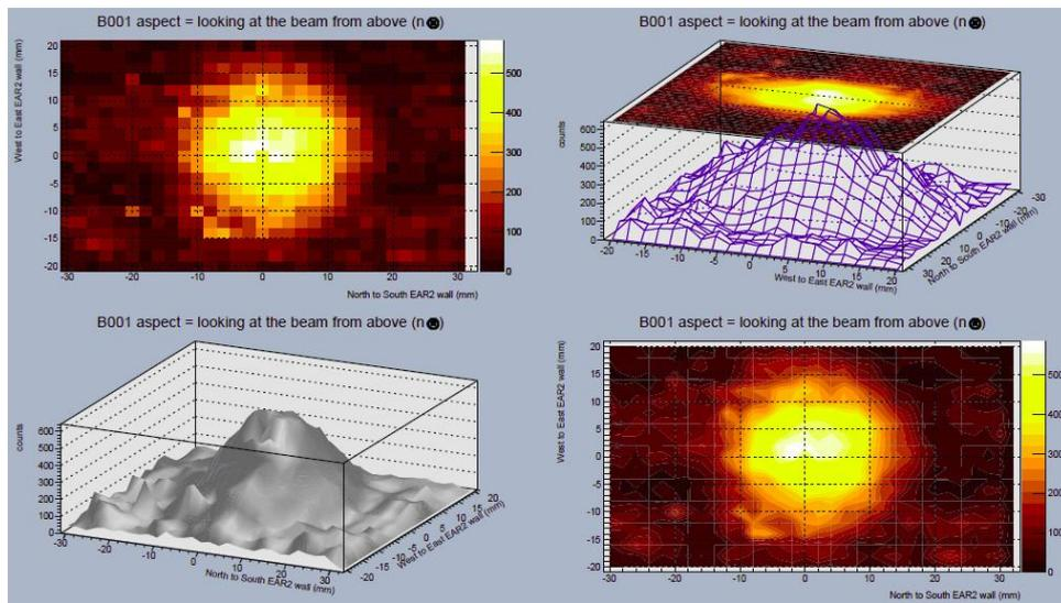
**Fig. 3.** Results from the short irradiation. Different aspects of the neutron beam spatial profile
