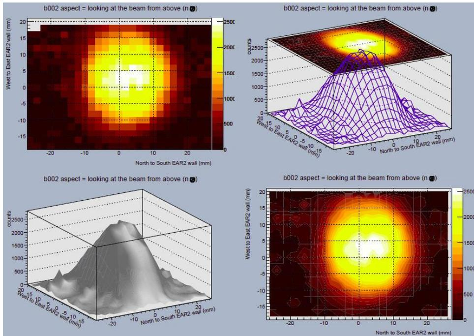
**Fig. 4.** Results from the long irradiation. Different aspects of the neutron beam spatial profile.
