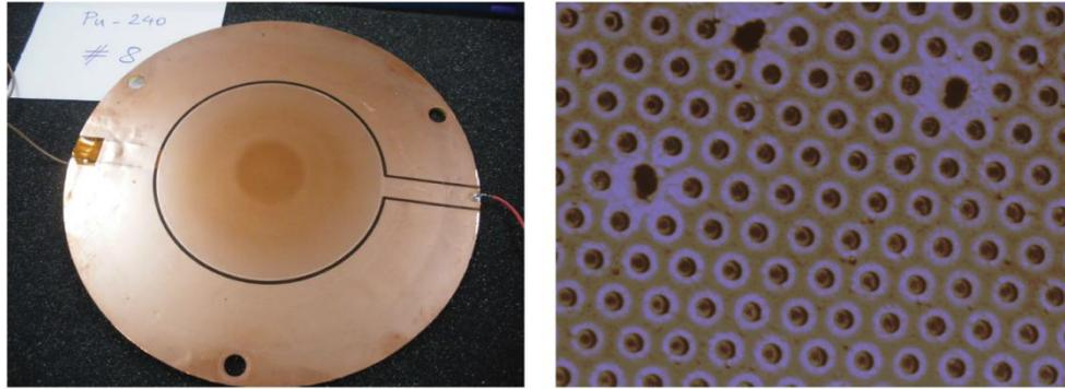
**Fig. 2.** Left: One of the Micromegas detectors used with a  $^{240}\text{Pu}$  sample pictured after the end of the measurement. A 3cm diameter discolouration is visible on the micromesh. Right: Picture of the micromesh taken with an electronic microscope. Mechanical damage around the rims of the holes can be observed. This leads to a severe deterioration of the detector gain and performance.
