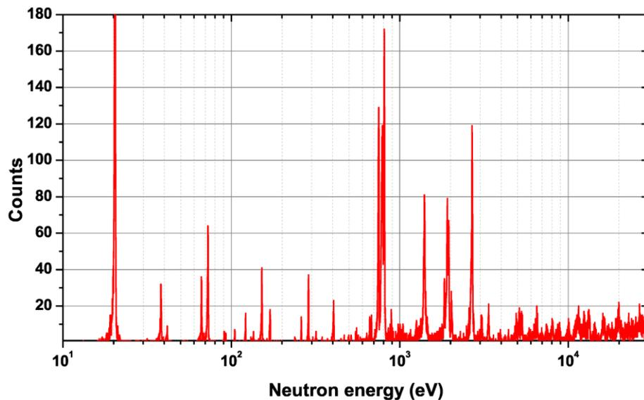
**Fig. 4.** Resonances observed in the measured fission yields from the three  $^{240}\text{Pu}$  samples, after subtraction of contributions from contaminants. Several resonance clusters, attributable to the coupling between Class-I and Class-II states, are visible, while resonances can be observed up to a few tens of keV. Data are shown with a binning of 2000 bins per energy decade.
