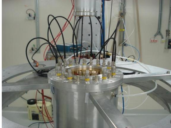
**Fig. 1.** A view of the chamber housing the samples and detectors, and the associated electronics placed in the neutron beam in EAR-2. The neutron beam arrives vertically from below and then continues in the vacuum tube above the chamber and onto the beam dump a few meters later. Approximately 15-20cm of air are present before and after the chamber.
