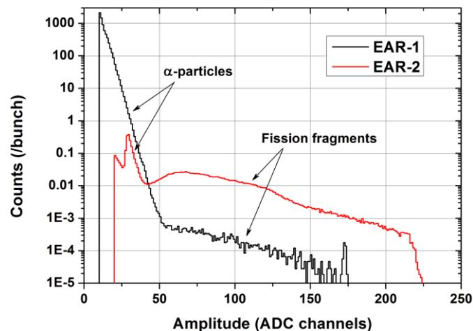
**Fig. 3.** Pulse-height spectra obtained from a  $^{240}\text{Pu}$  sample during the measurements in EAR-1 (black) and EAR-2 (red). Counts are normalised per beam bunch for direct comparison. The significant suppression of the sample-induced  $\alpha$ -background in EAR-2 is evident, as is the much higher rate of fission events.
