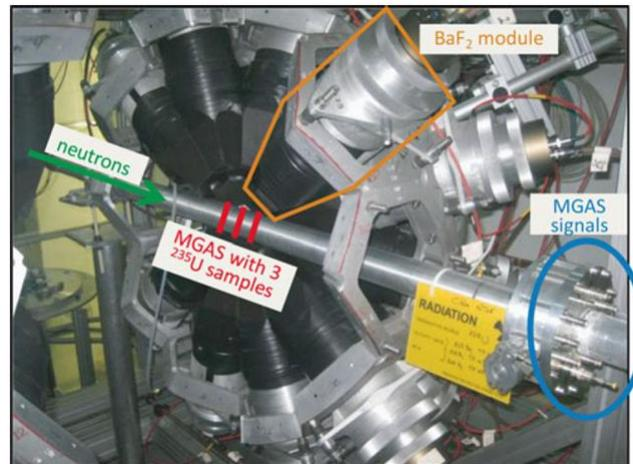
**Fig. 3.** A view of the “fission tagging” setup at n\_TOF with one hemisphere of the BaF<sub>2</sub> array and the chamber with the Micromegas detectors in the centre.
