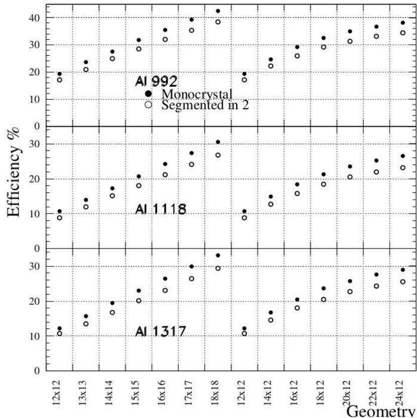
**Fig. 5.** Simulated sum-peak efficiencies for different detector geometries. On the geometry axis, the first number refers to the diameter of the detector and the second to its length, both measurements are given in inches. Full circle marks are for monocrystal detector, while the open circle ones correspond to a detector segmented in two parts.
