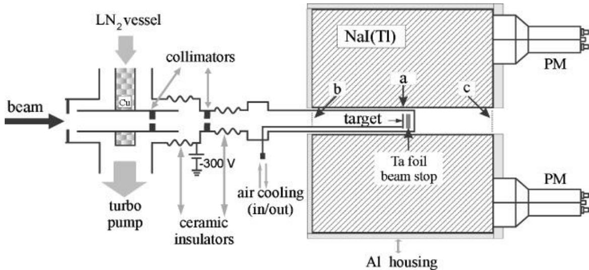
**Fig. 2.** Experimental setup at the Bochum university consisting of a 12x12 inch NaI(Tl) detector. The arrows marked with "a", "b" and "c" indicate target positions.
