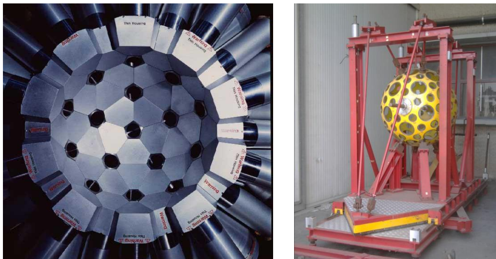
Fig. 7. Left panel: A picture of the BGO Ball installed at the Laboratori Nazionali di Legnaro. Right panel: A photo of the supporting frame.
