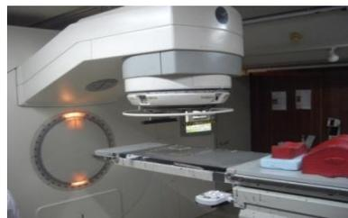
**Fig. 2** Medical Linac ELEKTA SL**Table 1** Characteristics of the irradiated foils
