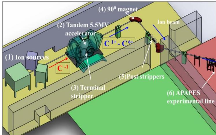
**Fig. 1.** The TANDEM accelerator laboratory of the NCSR “Demokritos” and the APAPES experimental station on the L30 beam line. The position of the three new strippers is indicated along the path of a carbon ion beam.
