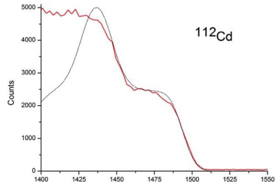
**Fig. 7** The RBS spectrum of <sup>2</sup>D beams on <sup>112</sup>Cd target
