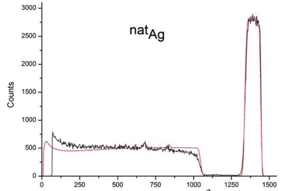
**Fig. 6** The RBS spectrum of <sup>2</sup>D beams on <sup>nat</sup>Ag target.
