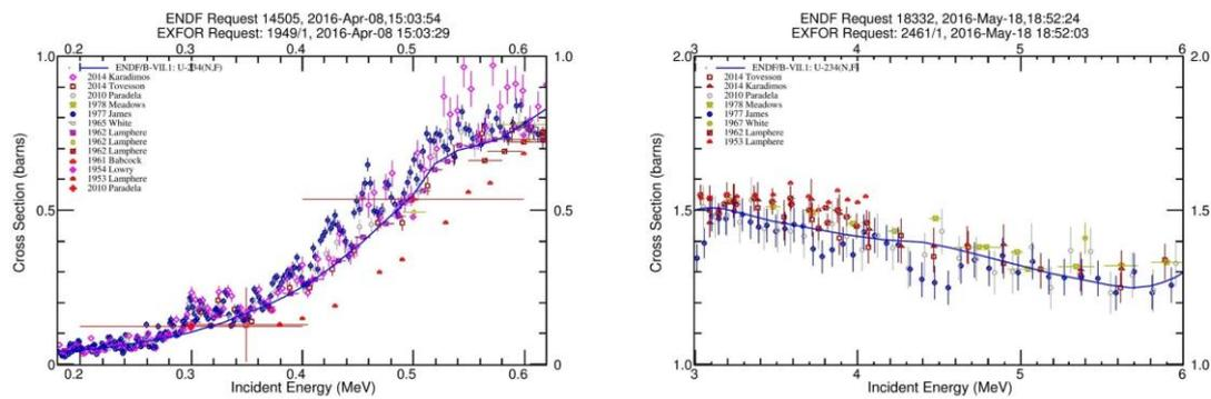
**Fig. 1.**  ${}^{234}\text{U}(n,f)$  cross section with both ENDF online evaluation library and experimental data. On the left the low-energy cross section is presented, while on the right the high-energy one
