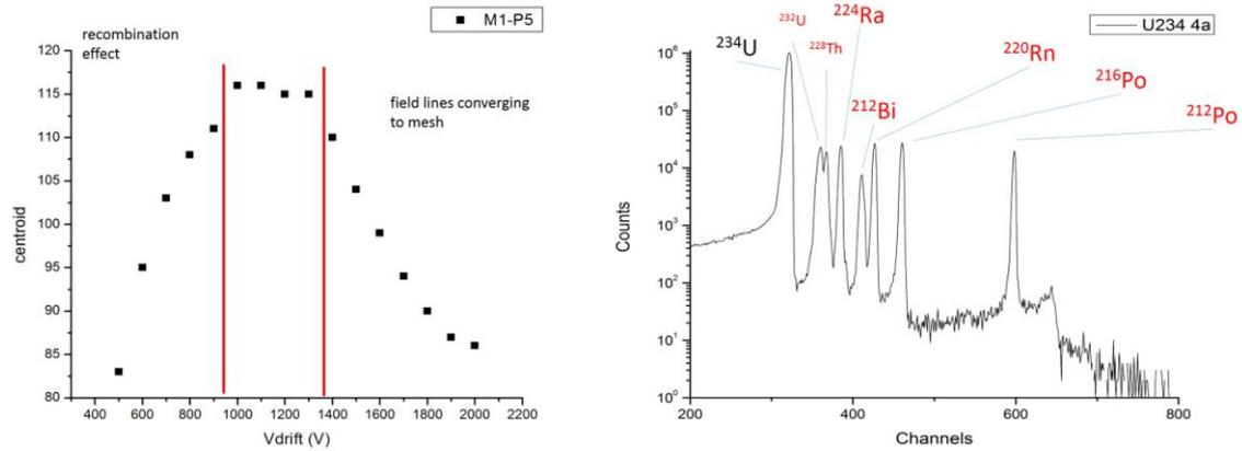
**Fig. 2.** Transparency curve of a MicroMegas detector (left).  $\alpha$ -particle spectrum of  $^{234}\text{U}$ , using a SSB detector. Impurities from the short-lived  $^{232}\text{U}$  and its decay chain are present in the target with a mass estimation of  $\sim 10^{-5}$  gr (right).
