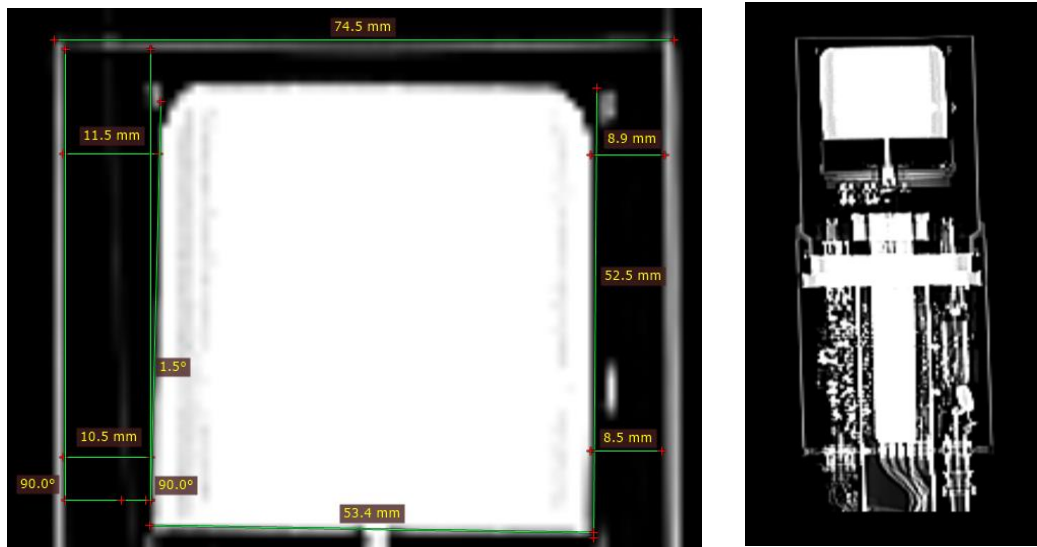
Fig. 9. Side (left) and full view (right) of the detector under X-rays in a medical CT scanner
