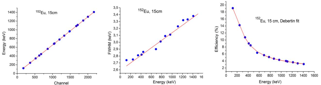
**Fig. 5.** Linearity (left), energy resolution (middle) and absolute efficiency (right) curves deduced from a  $^{152}\text{Eu}$  source placed at 15 cm from the detector's window and fitted with Debertin's equation
