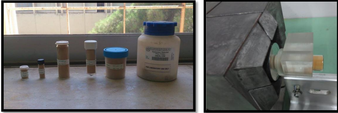
Fig. 1. The bulk samples and the IAEA reference material (left), and the set up (right)
